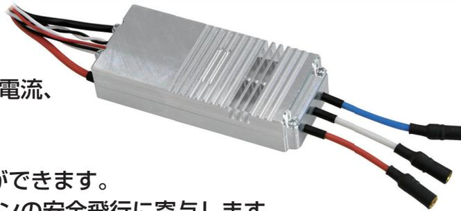
An electronic speed controller (ESC) dedicated to sensorless brushless motors. Compact and lightweight design with wide input voltage range and high output current supports high speed motor. Since the internal electronic components are moisture-proof, the ESC can be placed on the outside of the drone arm. It also has multiple built-in protection functions, which contributes to the safe flight of the drone.
